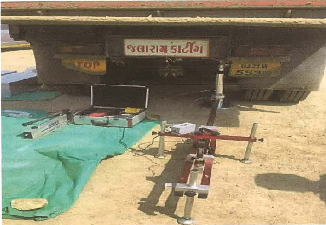
Fig. – 5 : E_{v2} Measuring Equipment
